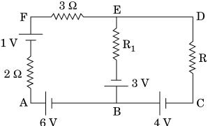
Use Kirchhoff's rules to determine the potential difference between the points A and D when no current flows in the arm BE of the electric network shown in the figure.
