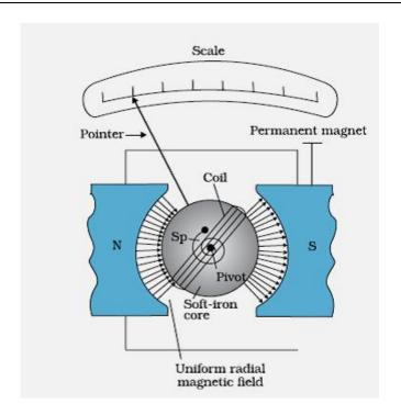
Principle: "Whenever a current carrying coil is placed in magnetic field, it experiences a deflecting torque."
