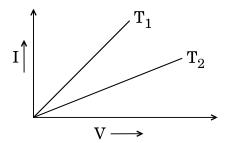
I - V graph for a metallic wire at two different temperatures,  $T_1$  and  $T_2$  is as shown in the figure. Which of the two temperatures is lower and why?
